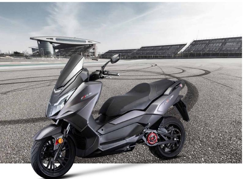
Interior Permanent Magnet, Brushless Motor Type Motor Power 3000 Watts 72V Rated Voltage Battery Type "ROTOM® Li-Ion Intelligent Integrated" 26/35Ah DualPower® Capacity(Ah) 15.5/18.6kg Battery Weight(kg) 80/100km Range(km) Charging Time(hour) 6-8 hours 1.5h Fast charing (hour) Charger Input(v) 110-220V Max Speed(km/h) 85km/h Disk Front Break Rear Break Disk 1820\*680\*1080mm Dimension(mm) 1300mm Wheelbase(mm) 130/60-13 Front Tyre 130/60-13 Rear Tyre N.W.(kg) 126kg
