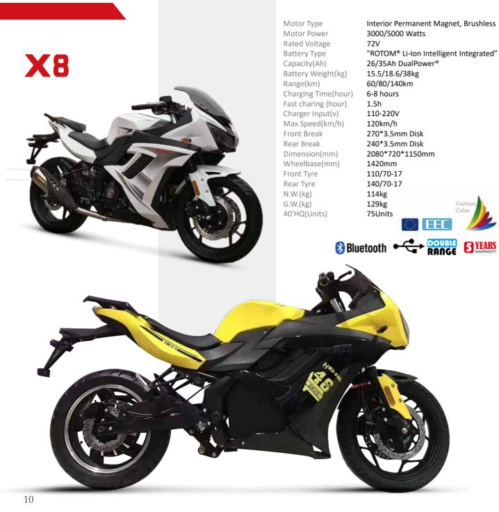
Motor Type Motor Power Rated Voltage Battery Type Capacity(Ah) Battery Weight(kg) Range(km) Charging Time(hour) Fast charing (hour) Charger Input(v) Max Speed(km/h) Front Break Rear Break Dimension(mm) Wheelbase(mm) Front Tyre Rear Tyre N.W.(kg) G.W.(kg) 40'HQ(Units)
